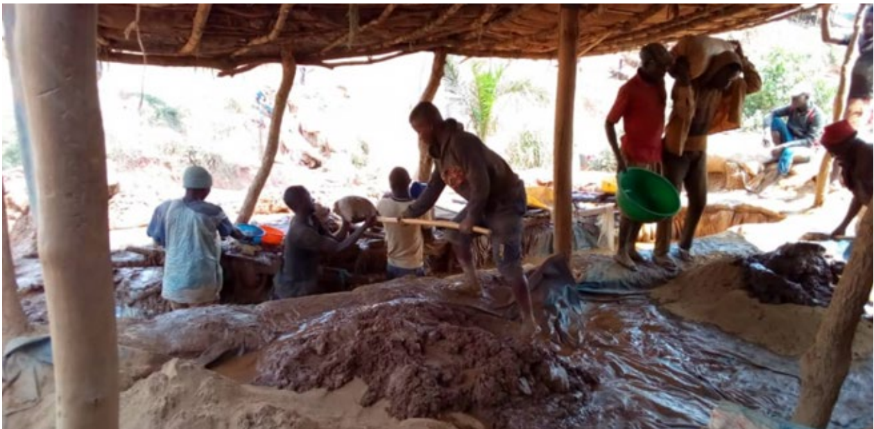
Picture 18: miners preparing mercury treatment of gold in a mine in Misisi, in the territory of Fizi, South Kivu
